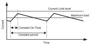
Inductor current operating in a "soft" overload
