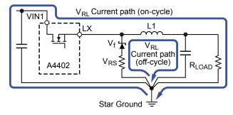
Figure 2. Current limiting during overload
