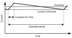
Figure 1. Current limiting during overload
