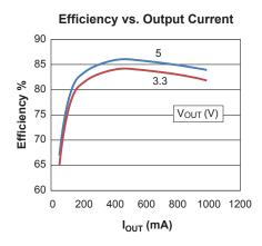
Data is for reference only. Efficiency data from circuit shown in left panel.
