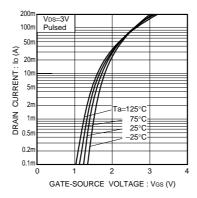
Fig.2 Typical transfer characteristics
