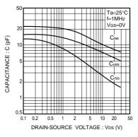
Fig.11 Typical capacitance vs. drain-source voltage
