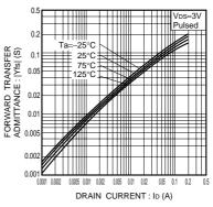
Fig.8 Forward transfer admittance vs. drain current
