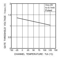
Fig.3 Gate threshold voltage vs. channel temperature
