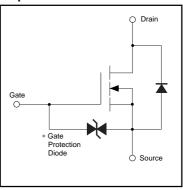
\*A protection diode is included between the gate and the source terminals to protect the diode against static electricity when the product is in use. Use a protection circuit when the fixed voltages are exceeded.
