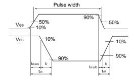
Fig.14 Switching time waveforms
