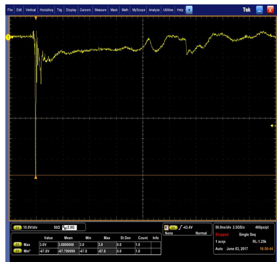
Fig2. ESD Clamping Voltage Screenshot Negative 8 kV Contact per IEC61000-4-2
