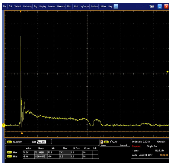
Fig1. ESD Clamping Voltage Screenshot Positive 8 kV Contact per IEC61000-4-2
