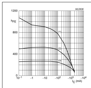
TR2 (PNP);  $V_{CE} = -5 \text{ V}.$
