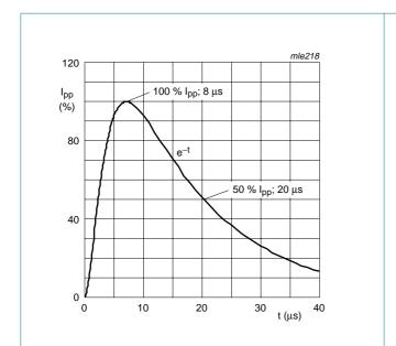
Fig 1. 8/20  $\mu$ s pulse waveform according to IEC 61000-4-5
