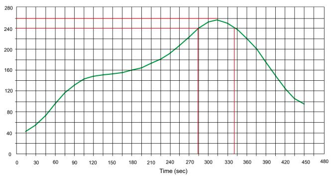
Peak Temp=257°C, Ramp Rate=0.802deg. °C/sec
