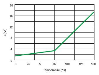
Fig 4.Typical Leakage Current vs. Temperature
