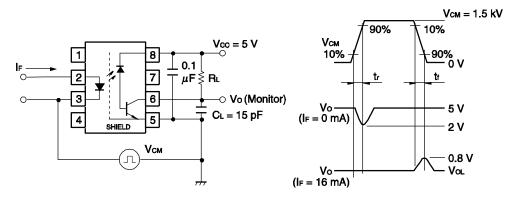
$\textbf{Remark} \quad \textbf{CL} \text{ includes probe and stray wiring capacitance}.$
