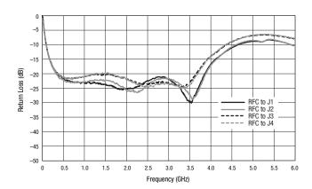
Figure 8. RFC Return Loss vs Frequency
