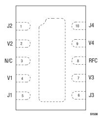
Figure 2. SKY13322-375LF Pinout – 10-Pin MLPD (Top View)
