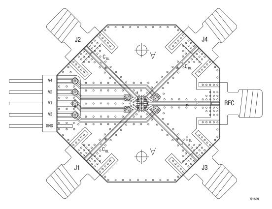
Figure 10. SKY13322-375LF Evaluation Board Assembly Diagram
