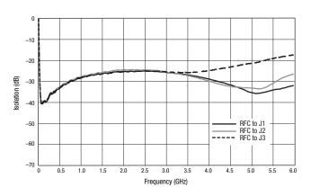
Figure 7. Isolation vs Frequency (RFC to J4 Insertion Loss State)
