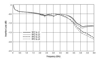
**Figure 3. Insertion Loss vs Frequency**
