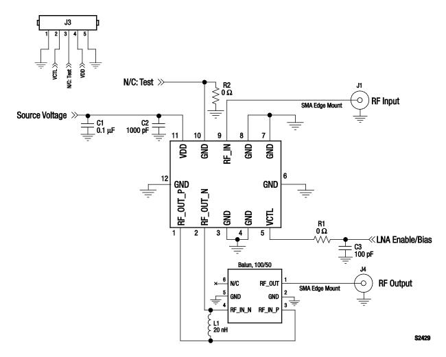
Figure 8. SKY65902-21 Evaluation Board Schematic
