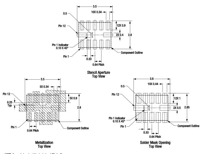
NOTE: thermal vias should be tented and filled with solder mask, 30-35 µm Cu plating recommended.
