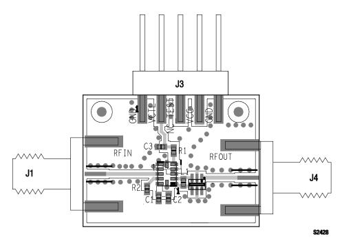
Figure 7. SKY65902-21 Evaluation Board Assembly Diagram
