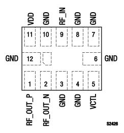
Figure 2. SKY65902-21 Pinout – 12-Pin MCM (Top View)
