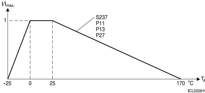
$$\text{Percent of } I_{\max} = 100 \left[ 1 - \frac{T_A - 25^{\circ}\text{C}}{T_{\max} - 25^{\circ}\text{C}} \right]$$
