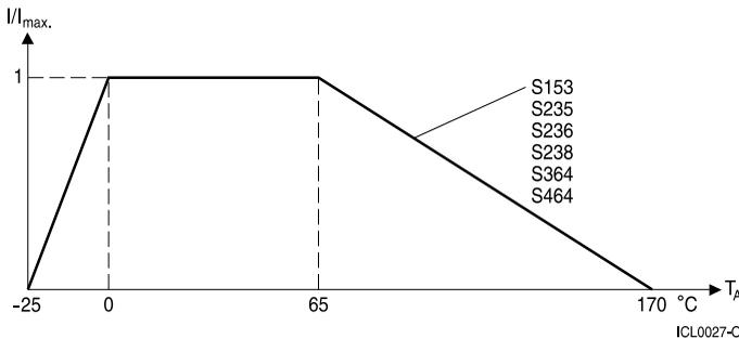
$$\text{Percent of } I_{\max} = 100 \left[ 1 - \frac{T_A - 65 \text{ }^\circ\text{C}}{T_{\max} - 65 \text{ }^\circ\text{C}} \right]$$
