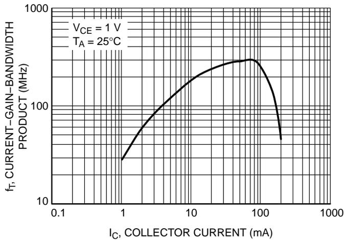
Figure 20. Current Gain Bandwidth Product vs. Collector Current
