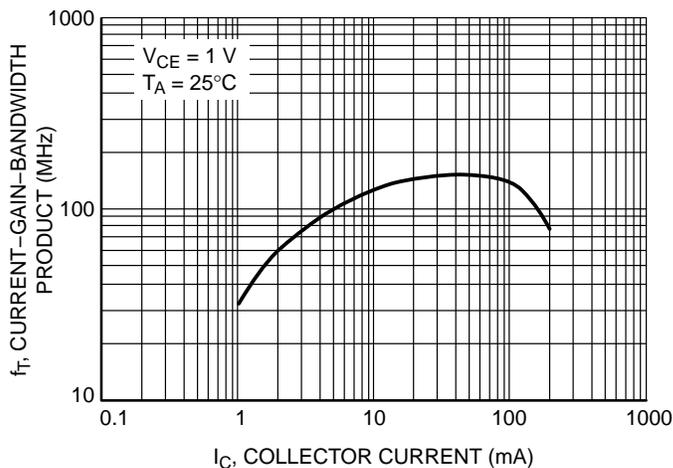
Figure 12. Current Gain Bandwidth Product vs. Collector Current
