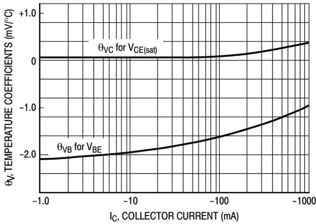
Figure 14. Temperature Coefficients
