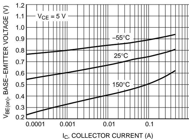
Figure 11. Base Emitter Voltage vs. Collector Current
