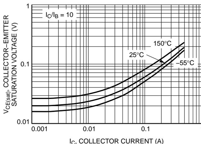
Figure 9. Collector Emitter Saturation Voltage vs. Collector Current
