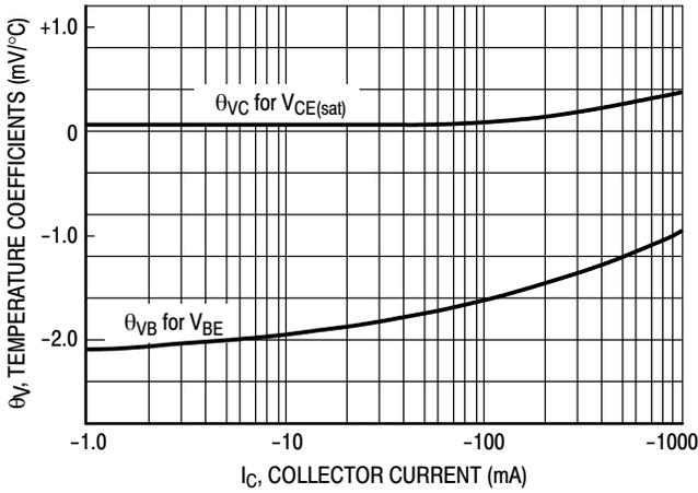
Figure 22. Temperature Coefficients
