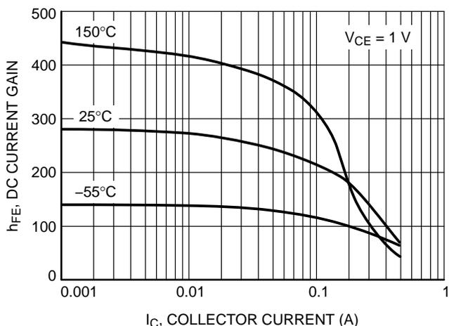
Figure 8. DC Current Gain vs. Collector Current
