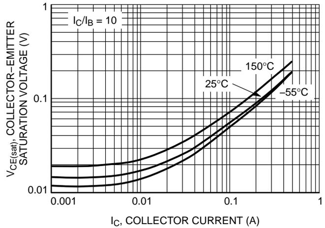
Figure 17. Collector Emitter Saturation Voltage vs. Collector Current
