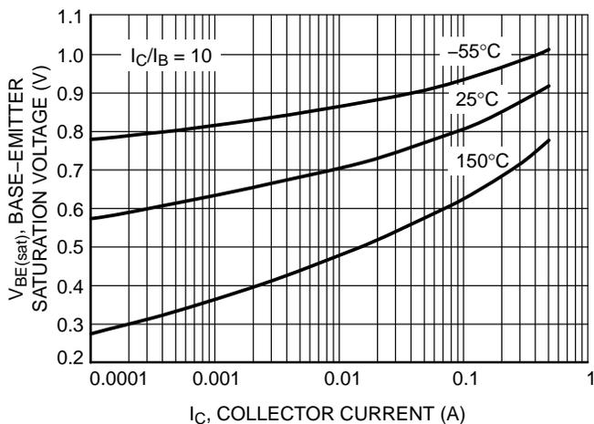
Figure 10. Base Emitter Saturation Voltage vs. Collector Current
