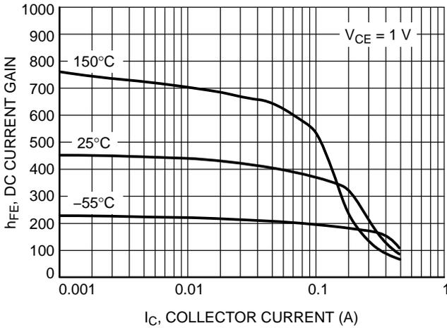
Figure 16. DC Current Gain vs. Collector Current
