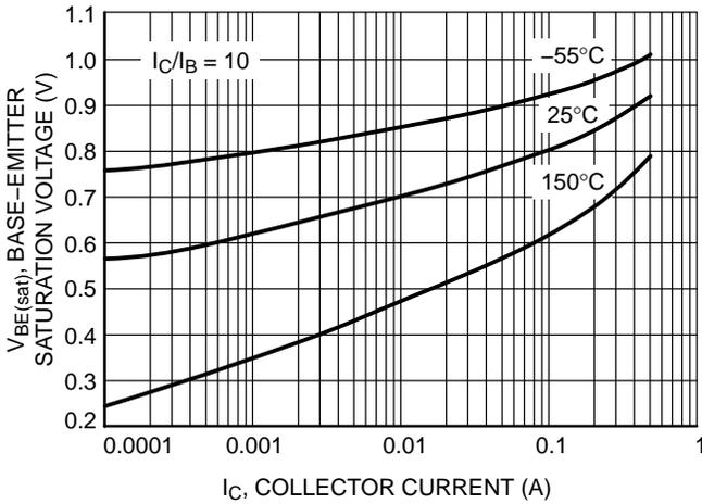
Figure 18. Base Emitter Saturation Voltage vs. Collector Current
