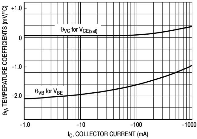
Figure 6. Temperature Coefficients
