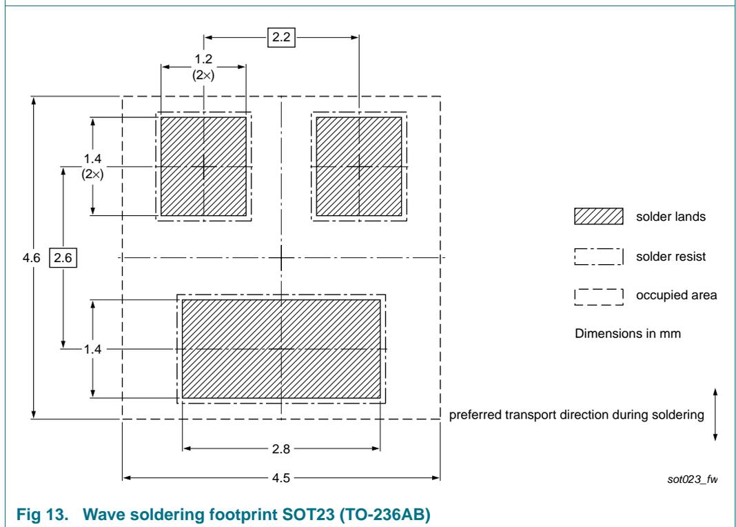
**Fig 13. Wave soldering footprint SOT23 (TO-236AB)**
