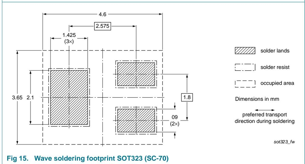
Fig 15. Wave soldering footprint SOT323 (SC-70)
