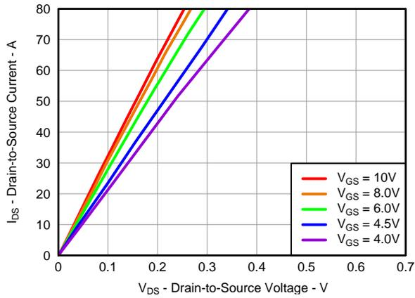
**Figure 2. Saturation Characteristics**
