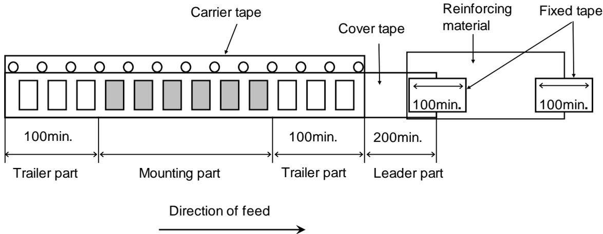
The cover tape shall not cover the sprocket holes
