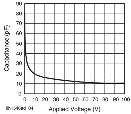
Fig. 5 - Switch Capacitance vs. Applied Voltage
