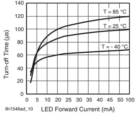
Fig. 10 - Turn-off Time vs. LED Current
