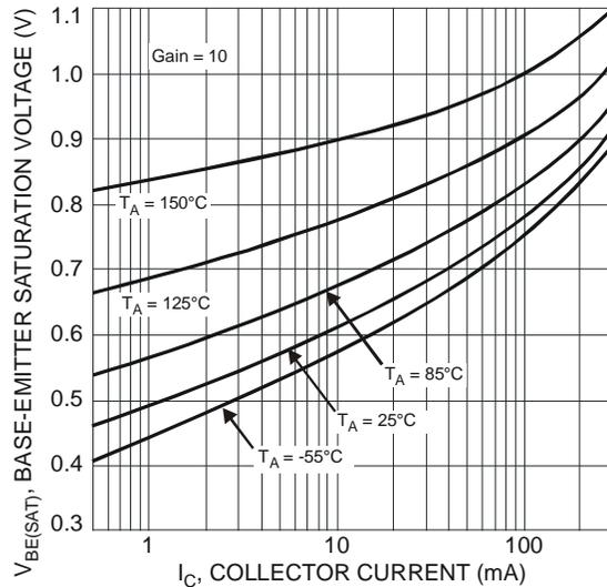
Fig. 9 Typical Base-Emitter Saturation Voltage vs. Collector Current
