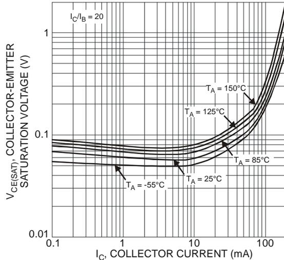
Fig. 7 Typical Collector-Emitter Saturation Voltage vs. Collector Current
