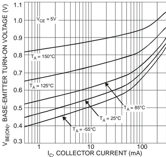
Fig. 8 Typical Base-Emitter Turn-On Voltage vs. Collector Current
