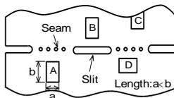
Products (A,B,C,D) shall be located carefully so that products are not subject to the mechanical stress due to warping the board. Because they may be subjected the mechanical stress in order of A>C>B≧D.
