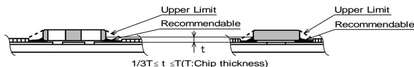
Accordingly increasing the solder volume, the mechanical stress to product is also increased. Excessive solder volume may cause the failure of mechanical or electrical performance.
