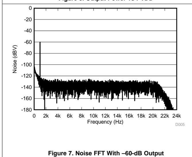
Figure 7. Noise FFT With -60-dB Output
