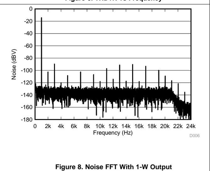
Figure 8. Noise FFT With 1-W Output
