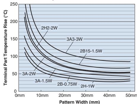
Room Temperature 25°C PCB: FR-4 t=1.6mm Cu foil thickness=35μm
